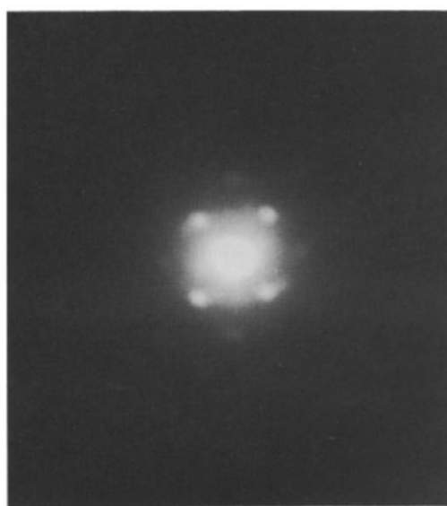
Figure 3 Low angle electron diffraction pattern of sample DB 7, tetragonal morphology
